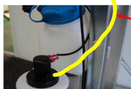
4 5 non-return valve from pump to atomiser waterhose from tank to Y-piece
